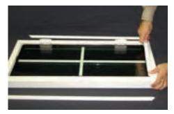
**5.** To reinstall, start with one of the shorter glazing beads. Place the mitered edge in the corner of the sash, paying special attention to insure the lower leg of the bead is tucked behind the ledge that the setting block is attached to. Snap in opposite corner in the same manner.
